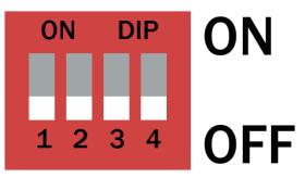
When the battery packs are connected in parallel, the dial code switch of each battery can be used to distinguish different Pack addresses. The hardware address can be set through the dial code switch on the board. The definition of the dial code switch refer to the following table:
